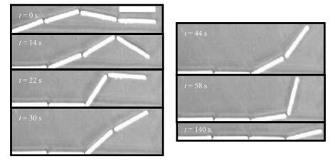
FIGURE 1. Snap-shots of the complex 'zippering up' motion for four connected candles at an air-water interface near a wall (at the bottom edge of each frame, just out of shot). The relevant Bond number here is  $B \sim 0.5$  and the scale bar represents 4 cm.
